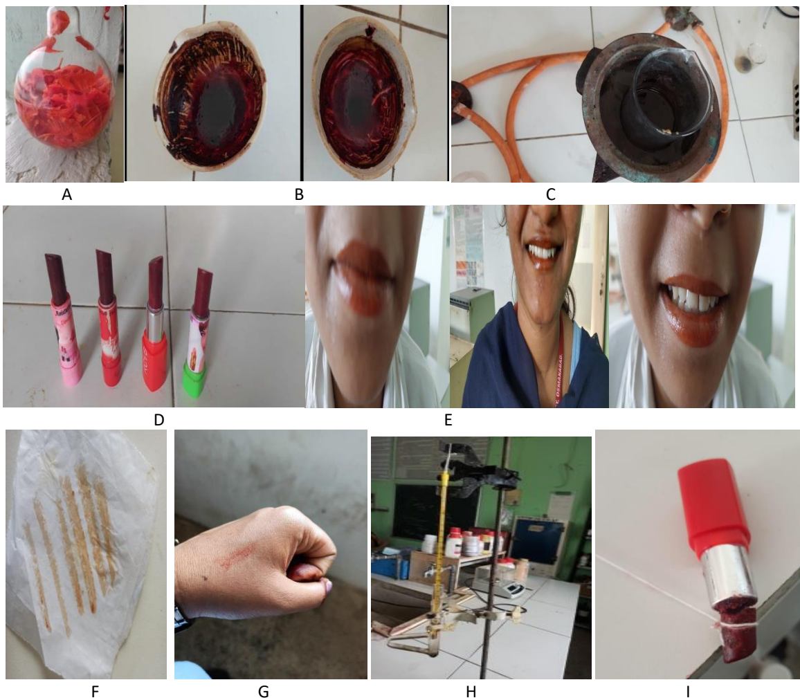
Figure 3: Events of Lipstick formation, A – Maceration, B- Concentrated extract, C- Water bath, D- Two lipsticks, E- Applicability, F- spread ability, G-consistency, H- Melting Point & I – Breaking Point
