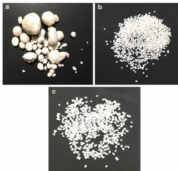
Figure 5: a) After spheronizing a formulation with a high-water content and longer threads, the result is an agglomerated product. b) After spheronizing a formulation with decreased water content and shorter threads, superior quality pellets are produced. c) Shows reasonable quality pellets of physical mixture formulation 4 .
