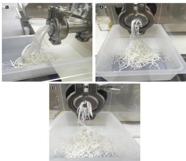
Figure 4: a) Denotes an extrudate of a high-water-content formulation with a high plasticity.
