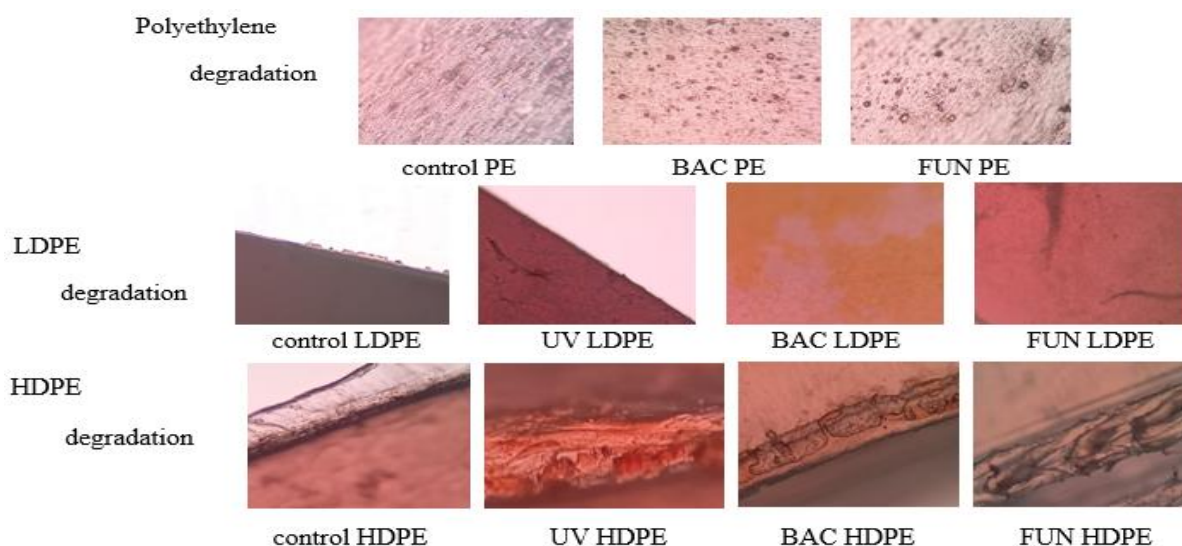
Figure 4: Microscopic imaging of polyethylene, LDPE, and HDPE (BAC 6 & FUN 1)
