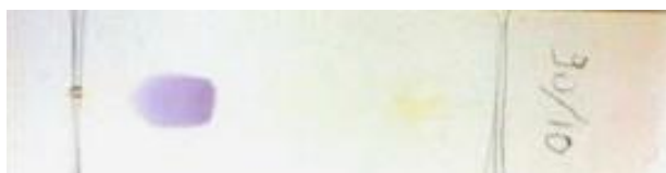
Figure 2: TLC is treated with ninhydrin, the presence of nicotine should yield a vivid purple coloration, indicating a positive result.
