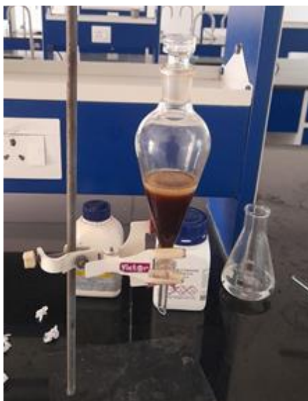
Figure 1: Extraction of nicotine from tobacco leaves using the partition coefficient technique
