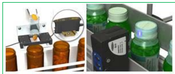
Figure 13: Sensor based packaging quality control
