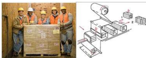
Figure 4: Stretch film wrapping
