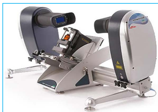
Figure 3: Laser diffraction system (spraytec, malvern) set up for nasal spray analysis.
