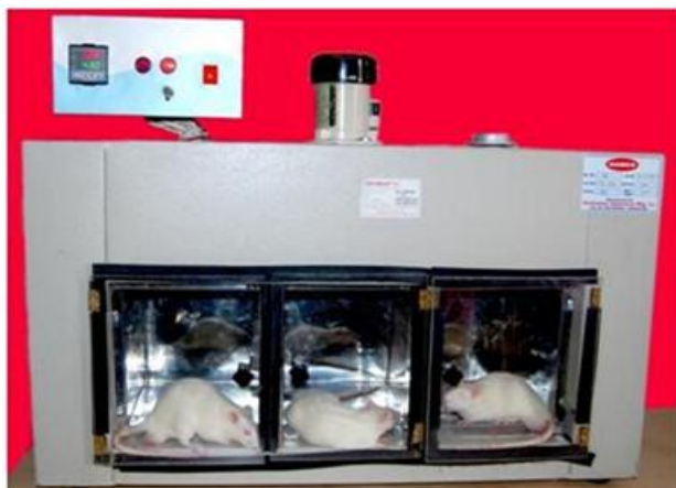
Figure 1: Incubator to maintain optimal temperature of 43°C and humidity of the atmosphere inside the compartments.
