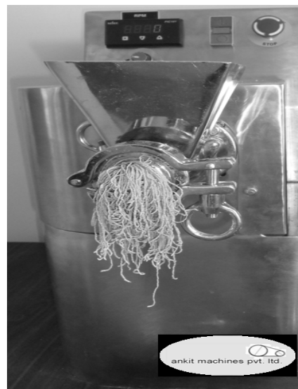
Photo 1: Single screw extruder machine; courtesy Ankit Machines Pvt Ltd, Nashik, (MS, India).
