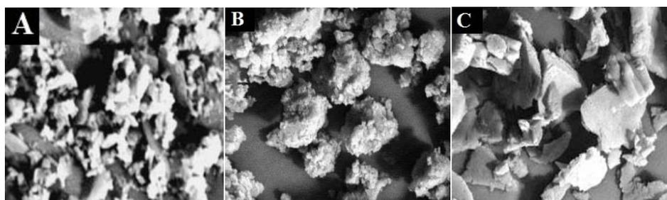
**Figure 4:** SEM microphotographs of (A) Pure domperidone, (B) PM of 1:9:0.25 domperidone/PVP K30/PL F-127 and (C) SD of 1:9:0.25 domperidone/PVP K30/PL F-127.
