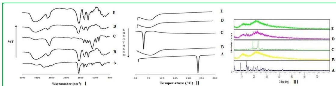
**Figure 3:** FTIR spectra (I), DSC thermograms (II) and PXRD patterns (III) of (A) Pure domperidone, (B) PVP K30, (C) PL F-127, (D) PM of 1:9:0.25 domperidone/PVP K30/PL F-127 and (E) SD of 1:9:0.25 domperidone/PVP K30/PL F-127.
