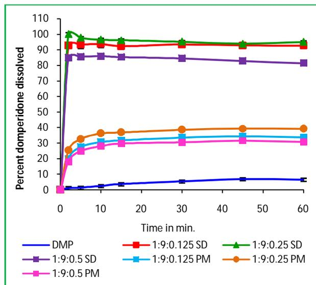
**Figure 2:** Dissolution profiles of domperidone from different domperidone/PVP K30/PL F-127 systems (SD: Solid dispersion and PM: Physical mixture) in phosphate buffer pH 6.8 at 37±0.5°C.
