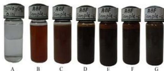
Figure 1: Optical photograph of Persea Americana A- 0.1 N AgNO 3 solution B- Leaf extract C- Leaf extract + AgNO 3 D- Leaf extract + AgNO 3 (After 30mins) E- Leaf extract + AgNO 3 (After 1 hr) F- Leaf extract + AgNO 3 (After 2 hrs) G- Leaf extract + AgNO 3 (After 24 hrs)
