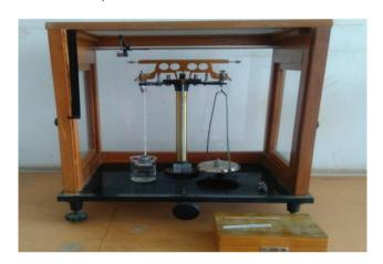
**Figure 1:** Modified physical balance for determination of bioadhesive strength of ocular insert
