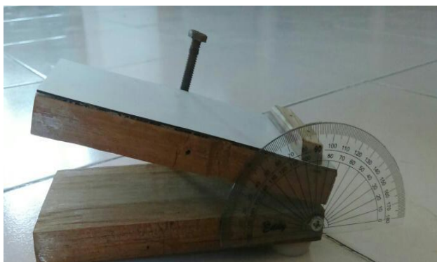
Figure 1: In- house lab-model for measurement of angle of slide
