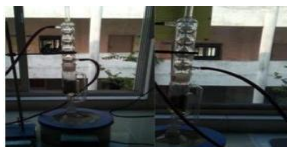
Figure 5: Soxhletation of P. pterocarpum leaf using water and ethanol
