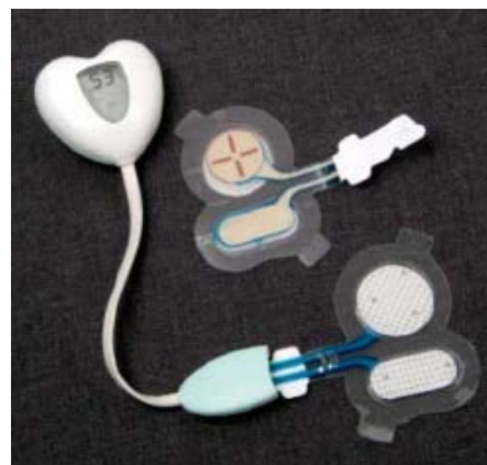
Figure 3: Vyteris iontophoretic device
