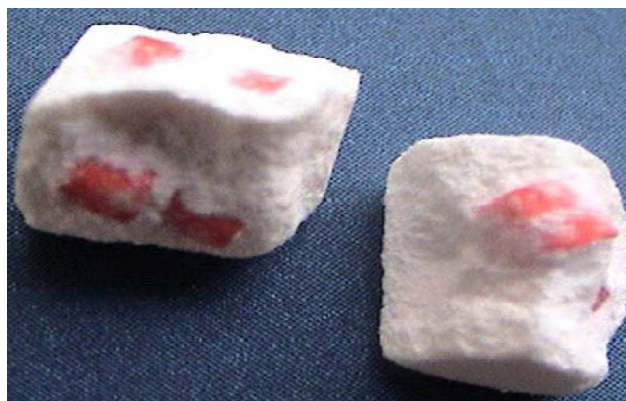
Figure 2: Fracture equatorial showing surfaces of the compressed mini-tablets system.
