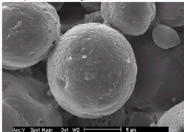
Figure 6(a): Scanning Electron Micrograph of optimized microcapsules at 20 x magnification.
