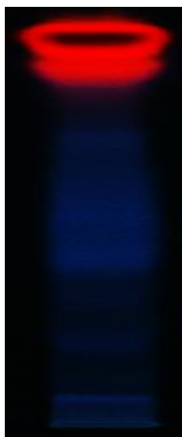
Figure 1: Different phyto-constituents of B. Lupulina ethanolic leaf extract at 366 nm on HPTLC plat with 10 \mu L of extracts.
