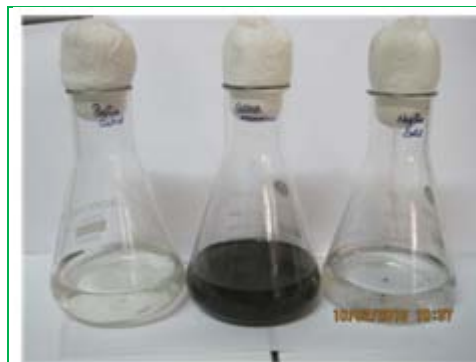
Figure 1: Image showing green synthesized Silver Nanoparticles with Positive Control, Test and Negative Control silver nanoparticles in the solution.
