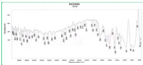
Figure 1: FT-IR spectra of desvenlafaxine Succinate
