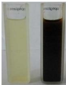
Figure 1: Solution containing FeSO 4 .7H 2 O before (left) and after (right) reduction with NaBH 4
