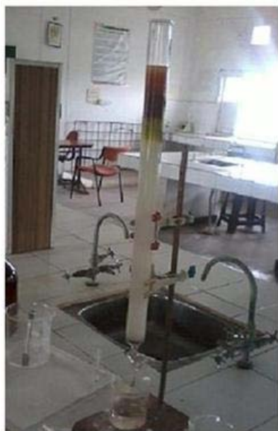
Figure 2: Movement of Mobile Phase in Column
