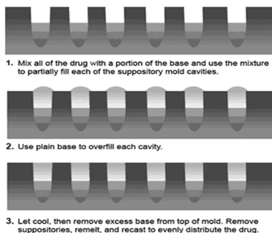
Figure 2: Double Casting Technique
