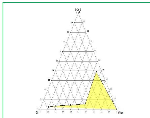
Figure 1: Pseudo ternary phase diagram with surfactant, co-surfactant ratio of 1:1
