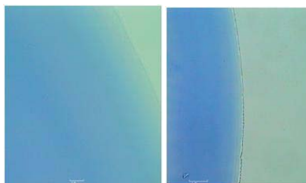
Figure 1: Appearance of film formed after application of gel a) under 40x magnification b) under 10x magnification
