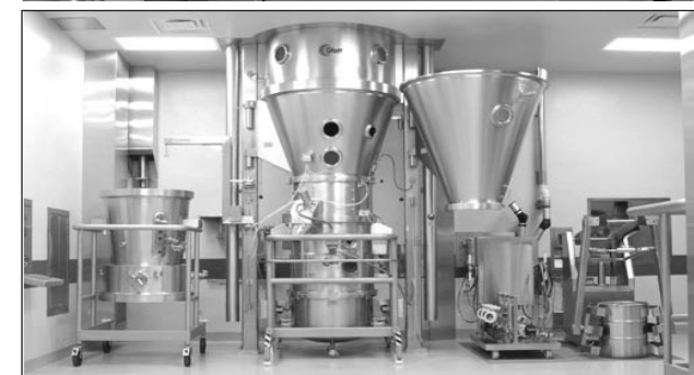
Figure 5: CPS™ pelletizing equipment- Lab scale and Production scale
