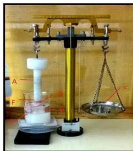
Figure 1: Modified mucoadhesion test apparatus (Fabricated)
