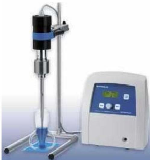
**Figure 4:** Probe Sonicator Used in Laboratory Scale for Preparation of NanoEmulsion
