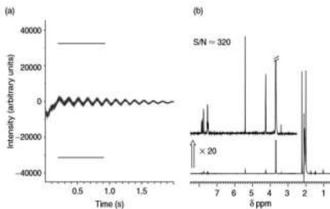
**Figure 6:** Optimized Receiver Gain with Solvent Signal Separation: (A) Free Induction Decay (B) Resulting NMR Spectrum
