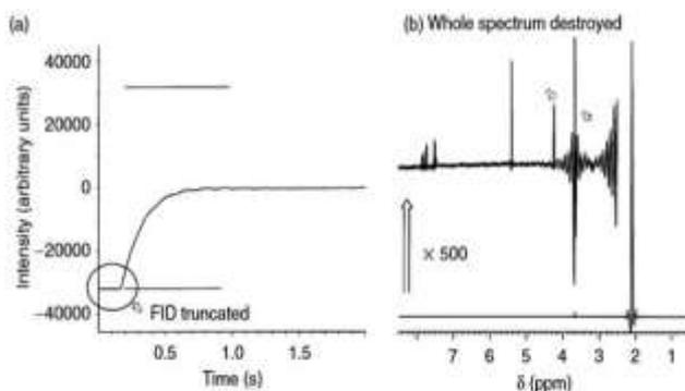
**Figure 5:** Increase In Receiver Gain Without Solvent Signal Separation: (A) Free Induction Decay (B) Resulting NMR Spectrum
