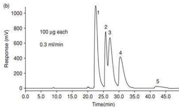
**Figure 3(B):** UV Chromatogram of the separation of Tocopherol Isomers with a 200 Fold Amount of Sample.
