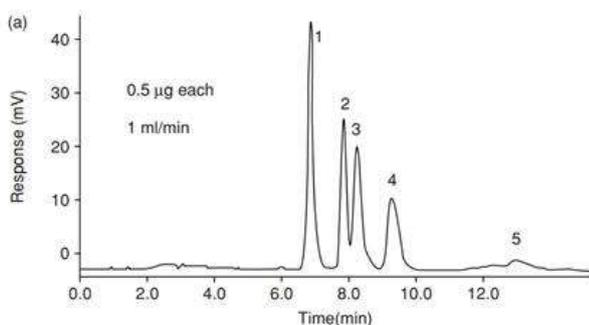
**Figure 3(A):** UV Chromatogram of the Separation of Tocopherol Isomers by Analytical Separation
