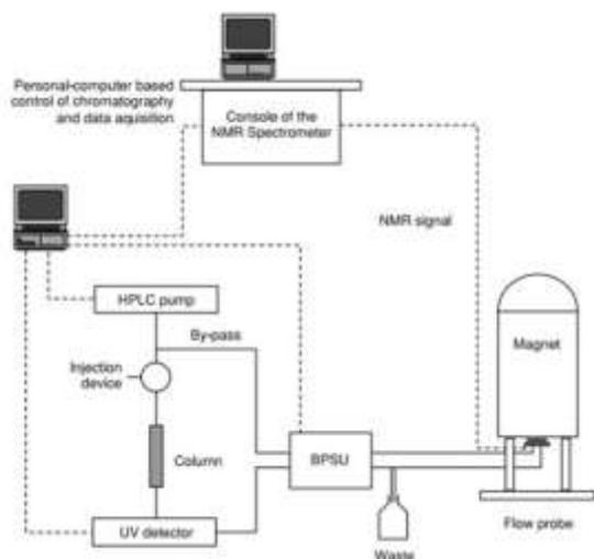
**Figure 2:** Schematic Diagram Of The Experimental Set-Up Used For LC-NMR Coupling: Bspu Bruker Peak Sampler Unit, (-) Capillary Junctions, (----) Electronic Junctions.
