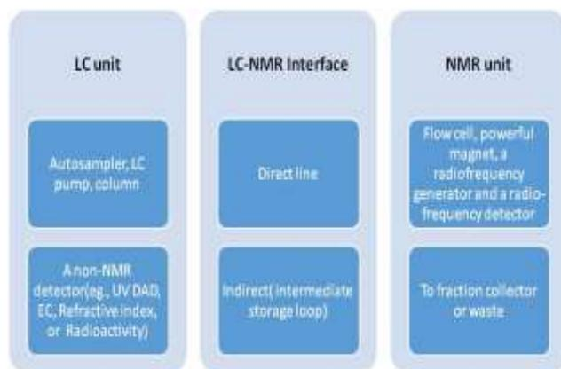
**Figure 1:** Instrumentation of LC-NMR
