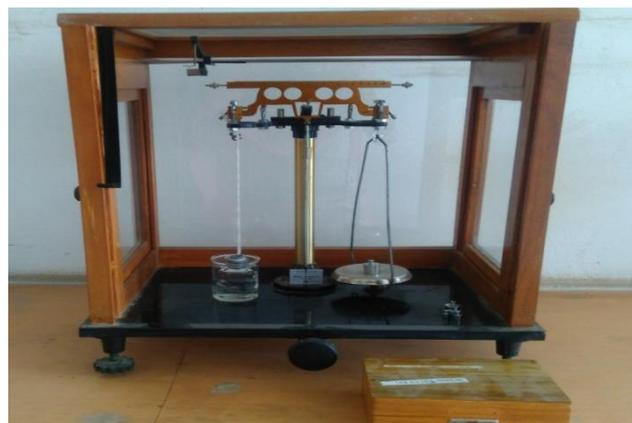
**Figure 1:** Modified physical balance for determination of bioadhesive strength of ocular insert
