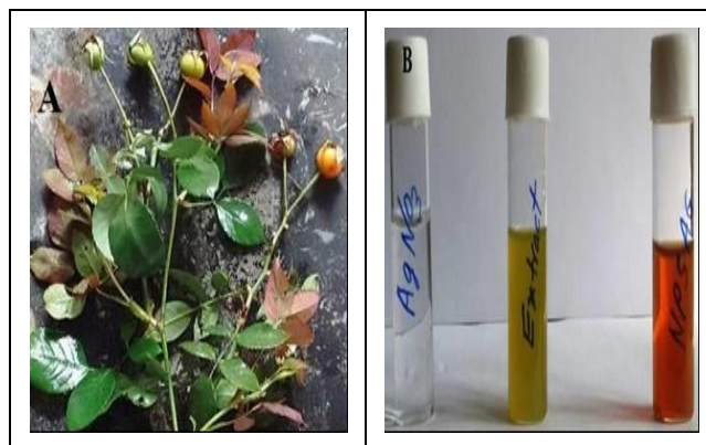
Figure 1: (A).Image of Rosa damascene hips, (B) Changing color intensity from yellow to brown of synthesized silver nanoparticles from extract of Rosa damascene hips
