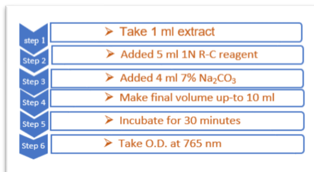
Figure 1: Process of estimation Total Phenolic content
