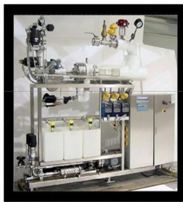
**Figure 1.** Advanced automatic Coating in Place (CIP) and Washing in Place (WIP) systems
