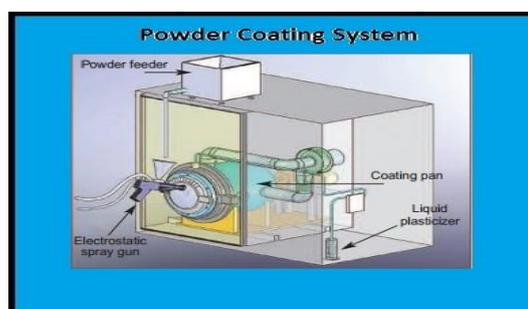
Figure 2: Electrostatic Powder Coating System<sup>16</sup>
