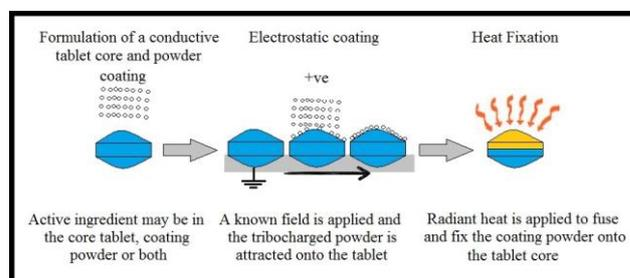
Figure 3: Schematic diagram of electrostatic dry coating.
