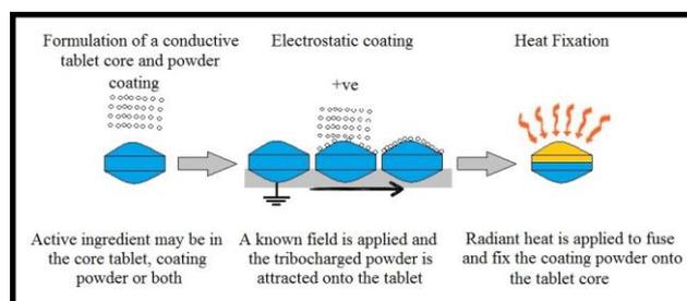
Figure 3: Schematic diagram of electrostatic dry coating.
