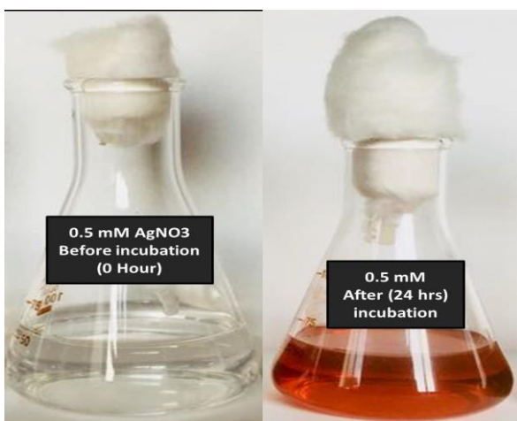
Figure 1: Synthesis of silver nanoparticles using ruta shoot extract (left – 0 hours) and (right – after 24 hours of incubation)
