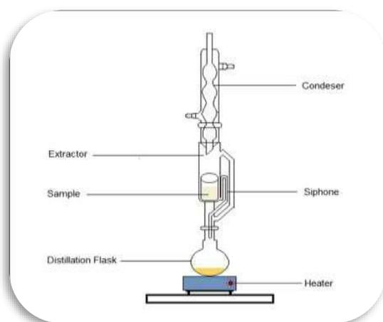
**Figure 1:** Extraction setup (Soxhlet extractor)
