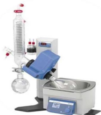
**Figure 2:** Rotary evaporator
