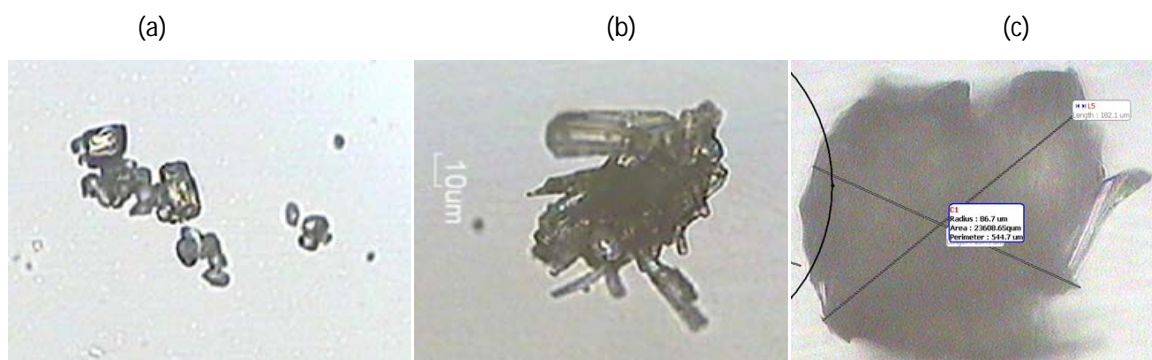
Figure 1: Micro images of – (a) original bulk powder MH; (b) Solvent change agglomerate powder MH-AG and (c) Wet granules powder MH-Wet
